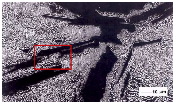
Fig. 3. Microstructure of hypereutectoid steel (Acerinox), laminated under hot conditions and normalised. The grain limits filled with continuous pro-eutectoid cementite as well as pearlite of thin interlamellar spacing inside the grains can be distinguished.
